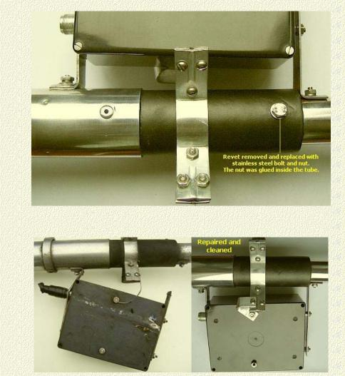
Due to the gap the antenna wobbled and one of the straps was broken. Shortcut I replaced a shortcut 27 pF cap with 4  $\times$  ceramic tube caps in series/parallel. e (iii) e «Back AØFR KB2LJJ Radio Mods Database
