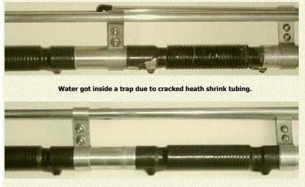
Cleaned and repaired coil
