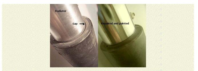
The antenna wobbled due to the gap caused by evaporation of the polyester. The tube was removed, the inside of the insulator applied with layers of 2 component polyester resin until a minimum variation of fit of the tube. Then I sanded the insulator for a perfect cylindrically curved shape and applied the last layer and placed the antenna back in the insulator. In fact the insulator was restructured to its original diameter.
