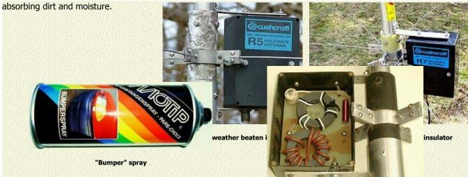
The insulator was "painted" with layers of 2 component polyester resin and sprayed (fig») with "bumper spray", a black car paint for polyester prevents the deterioration.
